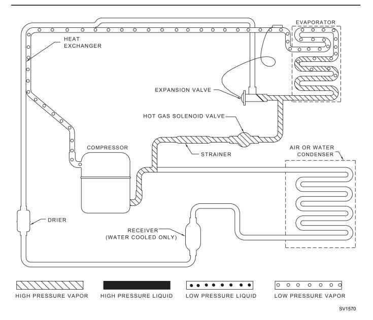
Figure 7-2. Self-Contained Harvest Cycle
